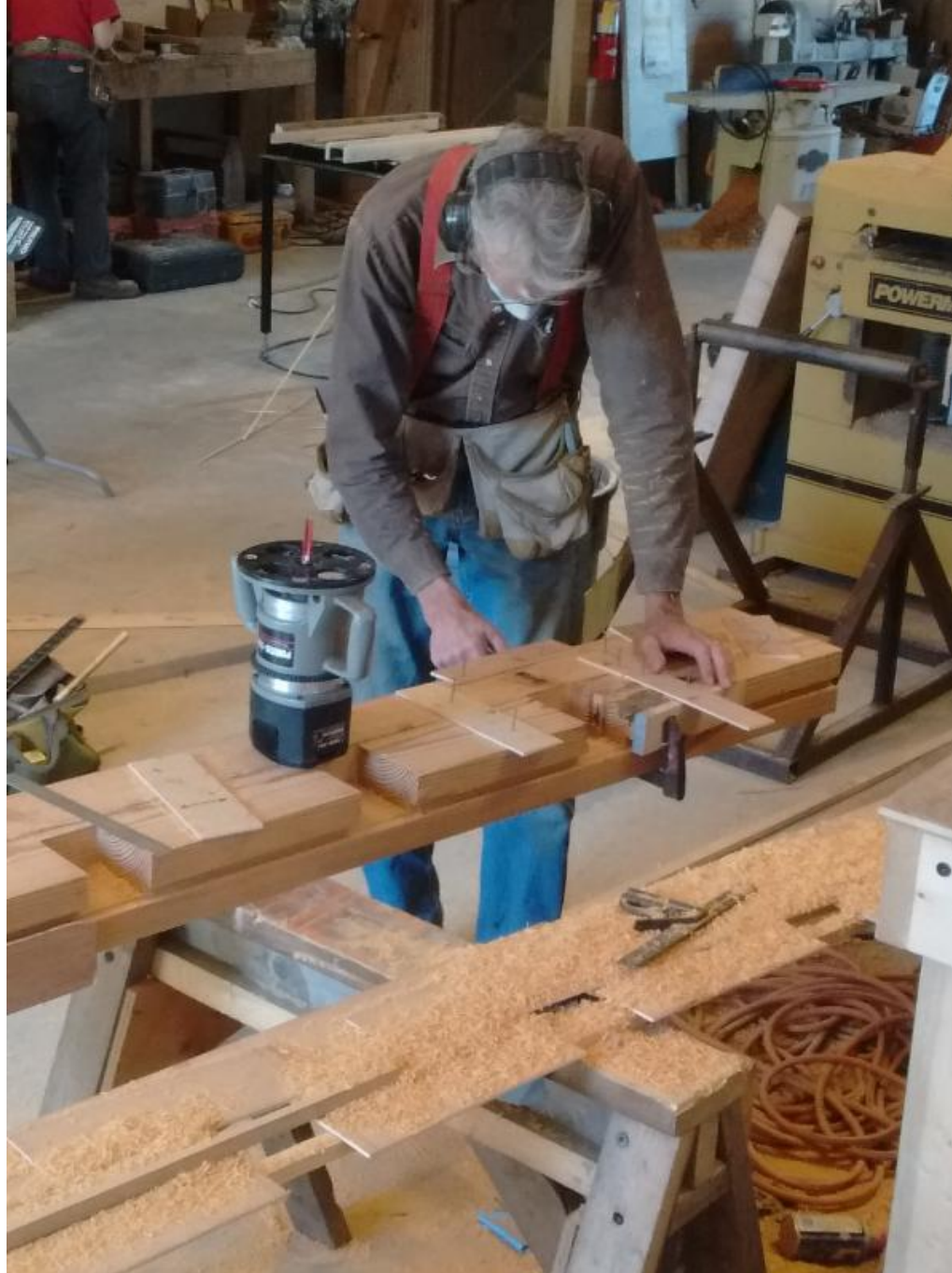
Shipwright, Jim Kricker works on a piece of the centerboard trunk.
