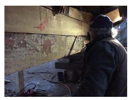
We made sure a thin bead of cotton was lined up between the bedlog and the keel before lowering the bedlog the final eighth of an inch.
