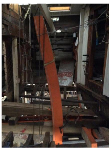
This photo shows the tail ledge, the vertical piece at the aft end of the centerboard trunk, being test fit into place.
