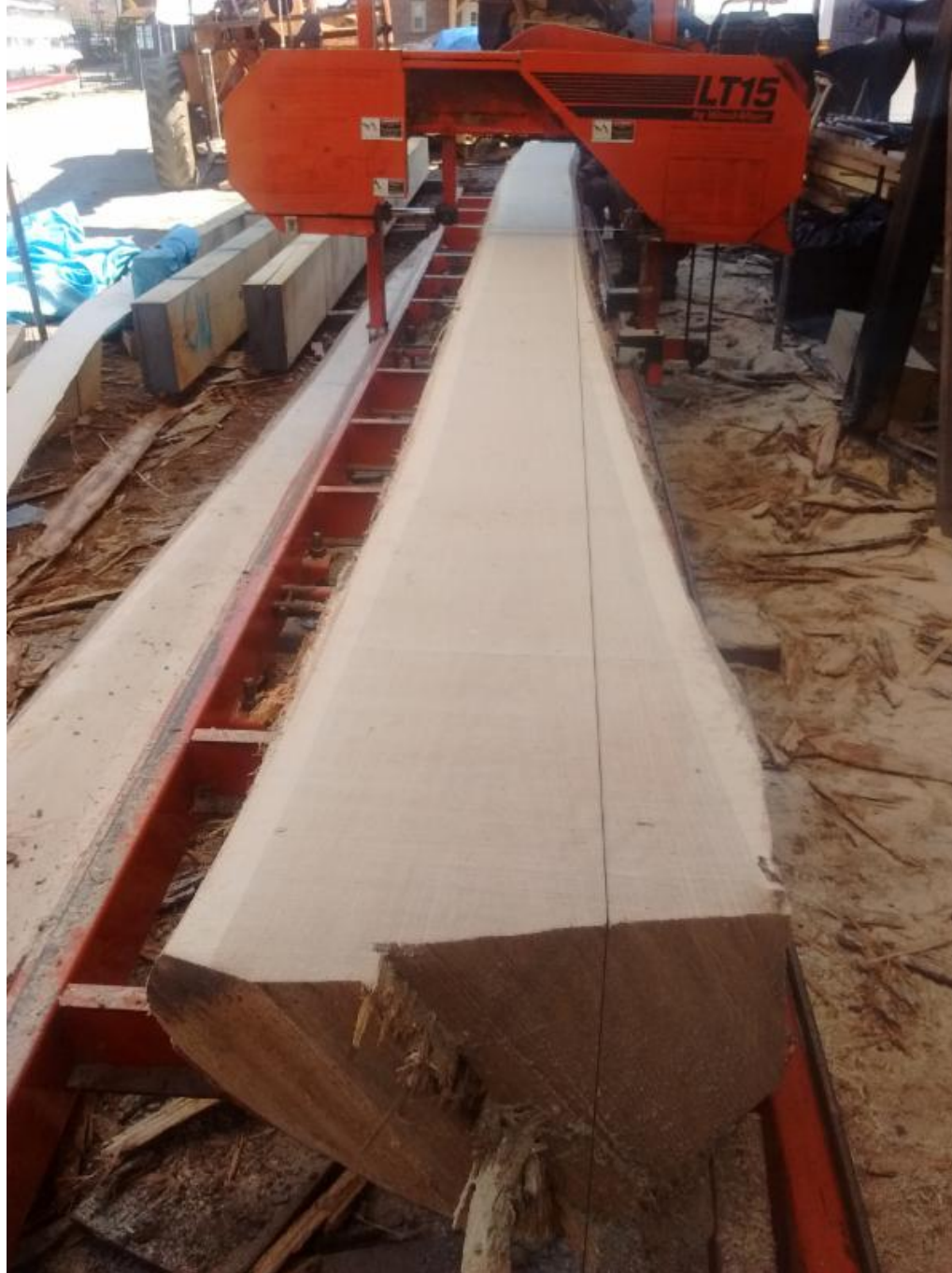
Wood being milled for centerboard trunk
