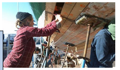
New hull planks
