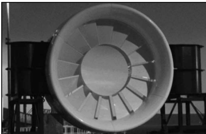
Open Hydro Turbine for generating free-flow tidal power
